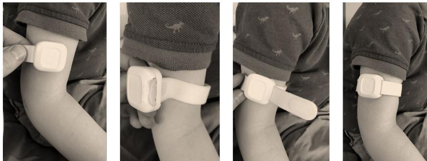
Figure 74: steps 4 to 7 of Gabi™ Band installation
