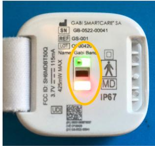
Figure 37: Green and red lights at the bottom of the sensor
